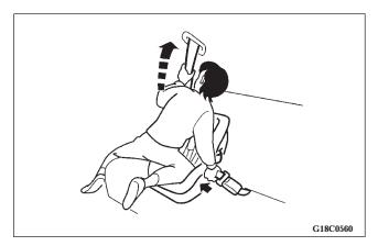
5. After confirming that the belt is locked, grab the shoulder part of the belt near the buckle and pull up to remove any slack from the lap part of the belt. Remember, if the lap part of the belt is not tight, the child restraint system will not be secure. It may help to put weight on the child restraint system and/or push on its seatback while pulling up on the belt (see illustration).
